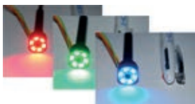
Microcirculation imaging device with LEDs and a small camera
