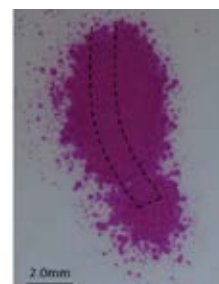
Analysis of cavitation of ultrasonically activated devices using pressure measurement film
